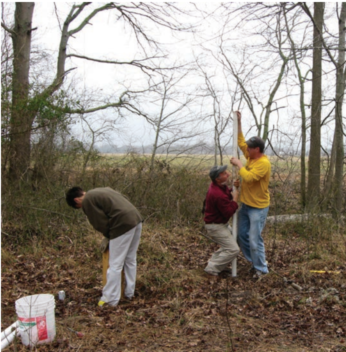
The installation of wells to monitor groundwater gives information about the concentration of nutrients in the groundwater. Photo by MCBP staff.
