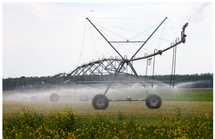
A central pivot irrigation system. Photo by Frank Liebig, Wikimedia Commons, CC BY-SA 3.0 DE.
